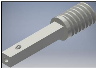
Image 1: New worm drive shaft design
